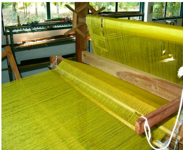
Loom fully threaded with silk yarn
